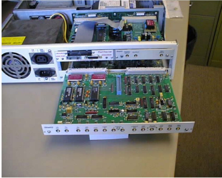
Figure 2.5 A photograph of the custom-made control board
