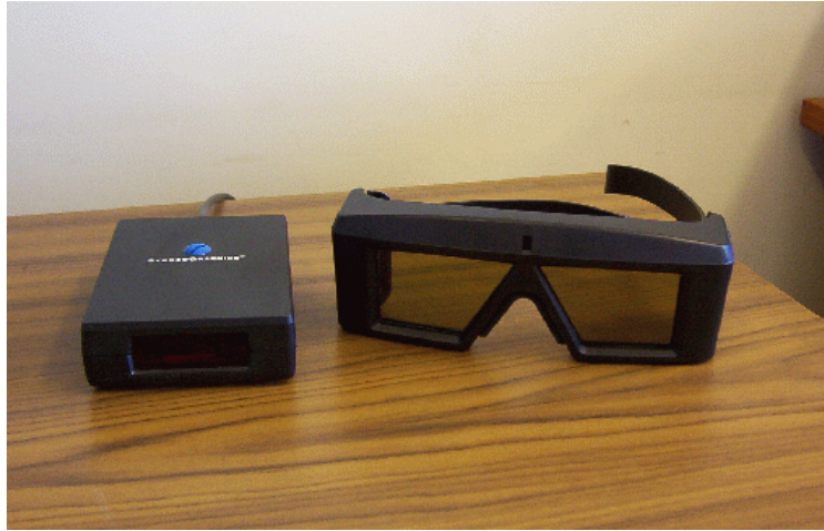
Figure 9: Stereo hardware: the emitter (left) and the stereo glasses (right).
