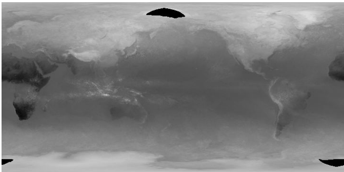
Figure 4: Cloud-free global image for 00.00 UT in January 1984, produced by taking maximum temperatures over a fourteen-day period at the same time each day.
